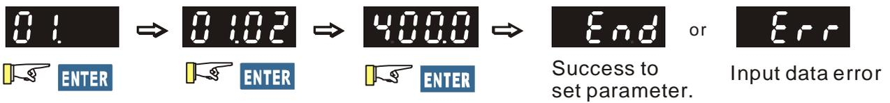
NOTE :In the parameter setting mode, you can press **ENTER** to return the selecting mode.
