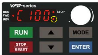
1000 ~ 9999 display: It will only display the first 3 digits. The LED at the bottom-right corner will light to indicate 10 times of the display value. For example, the actual value for the following figure is  $100 \times 10 = 1000$ .
