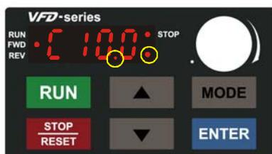
10000~65535 display: It will only display the first 3 digits. The LED at the bottom-right corner and the single decimal point between the middle and the right-most numbers will light to indicate 100 times of the display value. For example, the actual value for the following figure is  $100 \times 100 = 10000$ .
